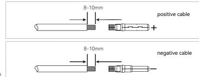
Figure 5.8 Striping off the insulation skin of cables
