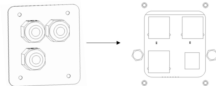
Step 2: Prepare a standard network cable and cable connector, then insert the network cable through the cable connector.
