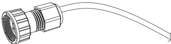
Step 3: Crimp the cable with a Rj45 plug which is inside of the cable connector.
