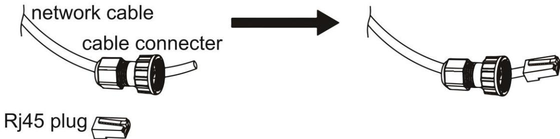
Step 4: Insert the cable connector into COM port at the bottom of energy station and screw it tightly. Then insert other side of the network cable into PC or another device.
