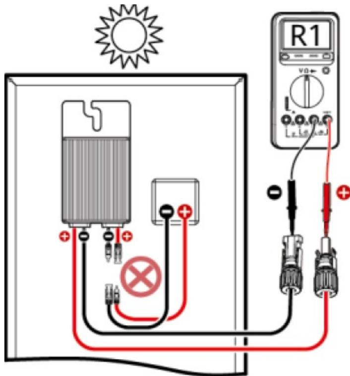
The optimizer output is connected to the PV module output:
