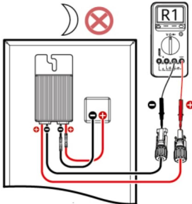
3. Check that the optimizer input is properly connected, and connect the output power cables to the optimizer. Measure the PV string resistance when the sunlight is sufficient.
