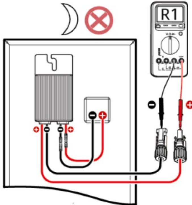
The optimizer input is not connected:  $1.1 \text{ k}\Omega < R1$
