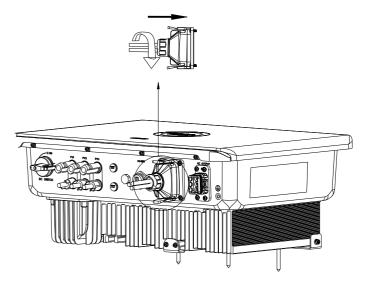
Figure 5.20 Securing sealing nut
