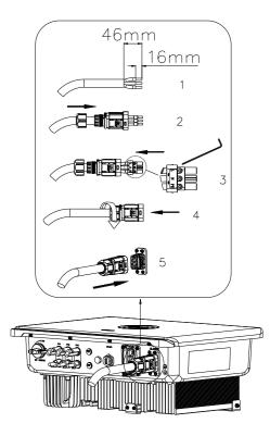
Figure 5.5 Connecting AC cable
