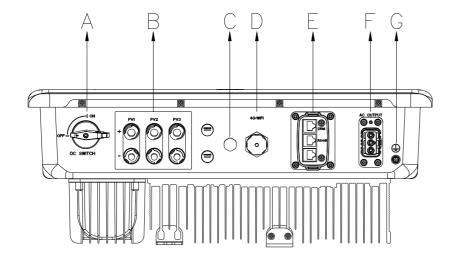
Figure 5.2 Electrical terminals of R6-5~10K-S3
