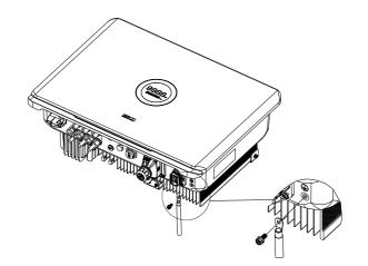
Note: Recommended conductor cross-sectional area of additional grounding cable is 6-16mm<sup>2</sup>.
