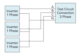
The inverter should not be installed in multiple phase combinations. If any such multiple inverter combination is not tested, it should not be used or external devices should be used in accordance with the requirements of AS/NZS 4777.1
