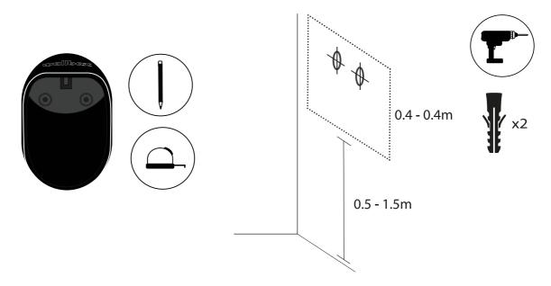
Insert the anchors screws into the fixing holes. Then secure the device to the walls by inserting and tightening the screws.
