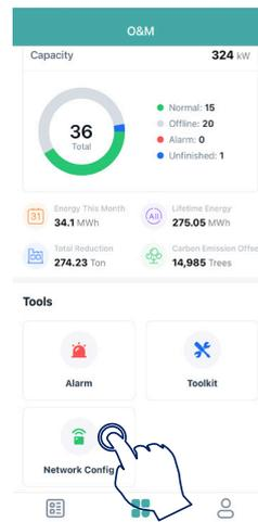
(b) Select the DTS's wireless network and click "Connect". (The network name of the DTS consists of DTS and product serial number, and the default password is ESS12345.)
