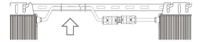
Use a Connector Protective Cap to make sure the unused AC connector to be closed.
