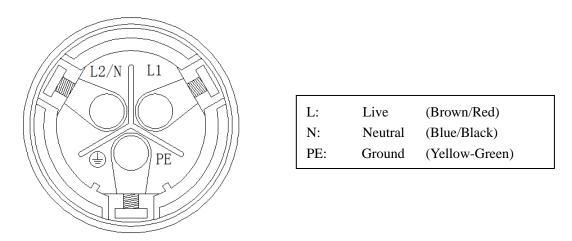
If the microinverter is connected to 120/240V split-phase power grid, connect two live lines to port L and port N.
