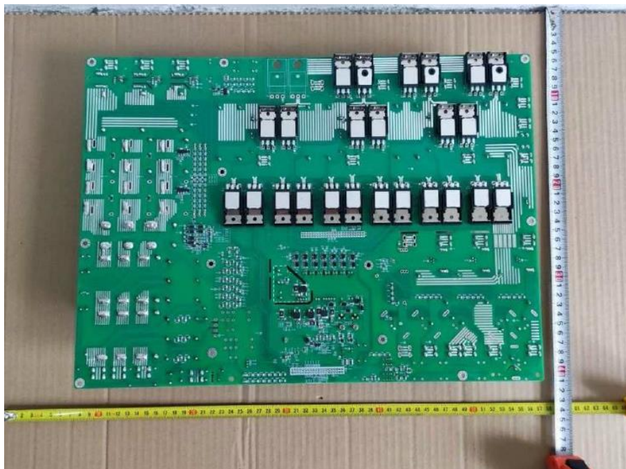
Back view of Main power board for R6-25K-T3-32, R6-30K-T3-32, R6-33K-T3-32, R6-36K-T3-32(DC side with varistor)
