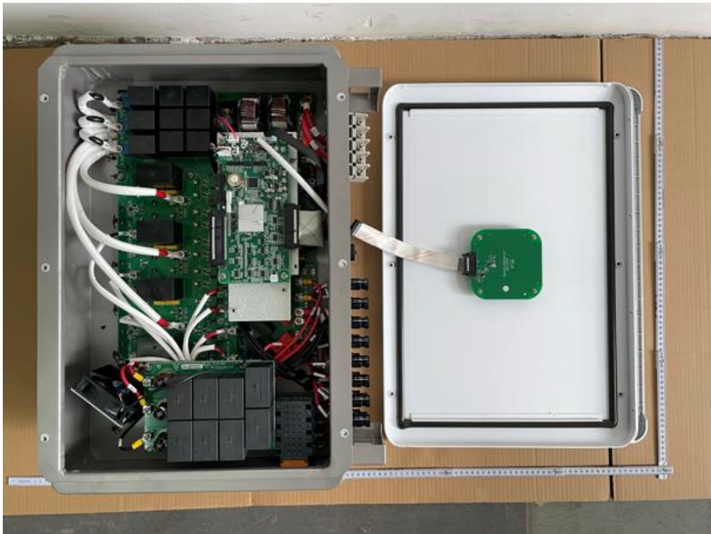
Internal view of R6-50K-T4-32, R6-40K-T4-32, R6-36K-T4-32
