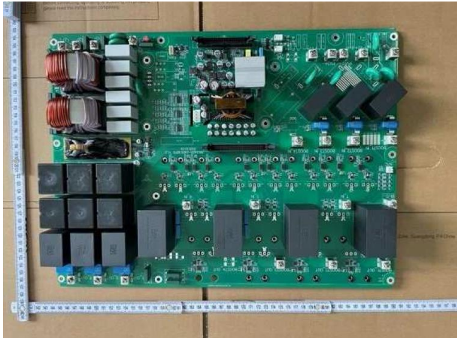
Front view of Main power board for R6-25K-T3-32, R6-30K-T3-32, R6-33K-T3-32, R6-36K-T3-32 (DC side with varistor)
