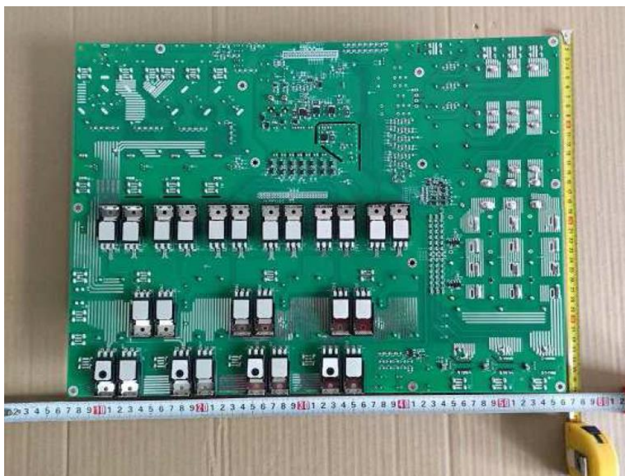
Back view of Main power board for R6-36K-T4-32, R6-40K-T4-32, R6-50K-T4-32 (DC side with Surge Protector version)
