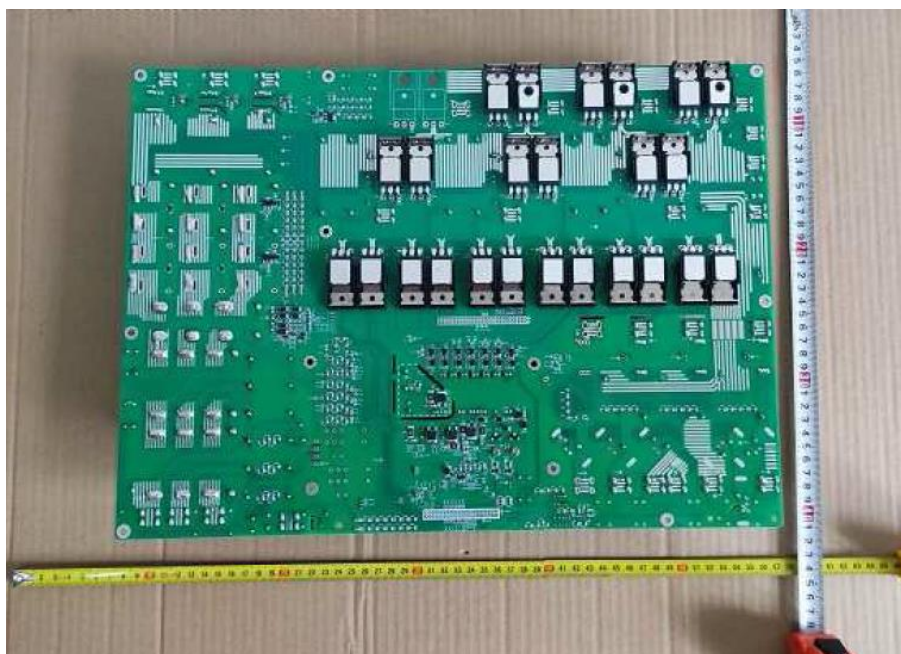
Back view of Main power board for R6-25K-T3-32, R6-30K-T3-32, R6-33K-T3-32, R6-36K-T3-32 (DC side with Surge Protector version)
