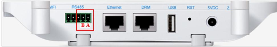
**Scenario 1:** If there is only one DTU in one system, when the RS485 cable length is more than 200 meters, we would recommend shorting jumpers on the two terminals on the left of the RS485 port.
