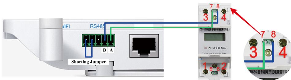
**Scenario 2:** When there are multiple DTUs in one system, please connect them one by one (as shown in the diagram below). The two shorting jumpers on the left of the on the last DTU will be recommended if the distance between microinverter and the last DTU is more than 200 meters.
