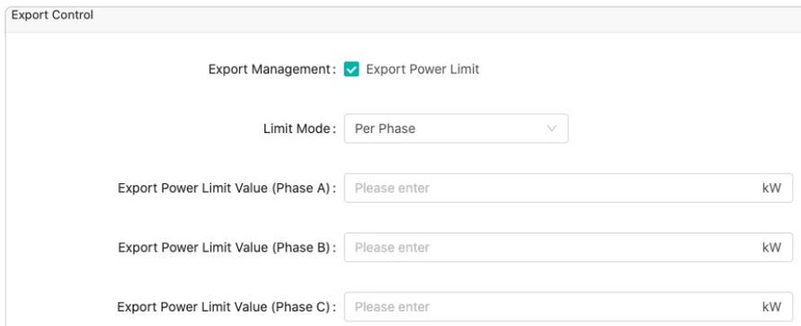
The following examples display twelve hoymiles HM-1500 4-in-1 microinverters connected to a three-phase system. The phase voltage is 230V and the maximum continuous output AC power of this system is 18kW. The output power of all the PV modules is 20kW. Each phase has four microinverters with maximum AC power of 6kW. Each example shows how the export power and solar power are affected under different conditions.
