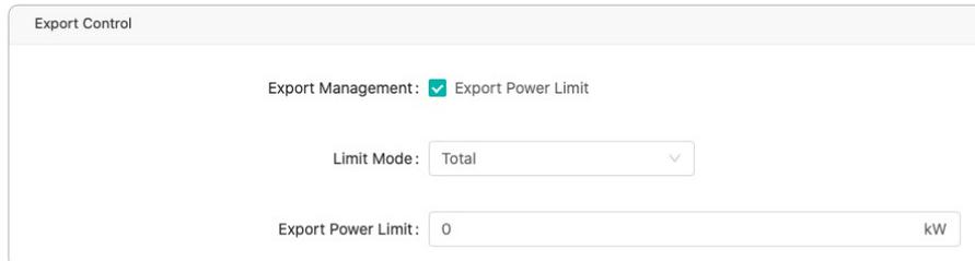
Per Phase (Only for three phase 230V/400V PV system): When you select “Three Phase 230V/400V”, which means the outputs of PV microinverters are connected to phase voltage, Per Phase can be selected and you can enter limit value of each phase. Export power of each phase will be limited to the value as shown in the picture below. The total export power is the sum of the PV production minus the load consumption of each phase.
