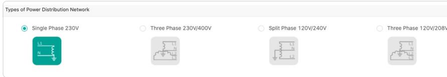
For “Three Phase 230V/400V”, the Limit Mode in Export Control contains two modes, namely Total and Per Phase Limit Mode, while for the other three types, there’s only Total Limit Mode.
