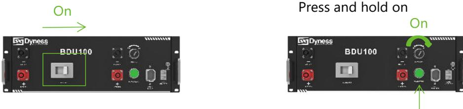
2 clusters HV4 usage: Turn on the circuit breaker on HV4 BDU100, turn on the power switch, and press hold the 'wake up' button for 10 seconds. Next, turn on the second cluster of batteries in order.
