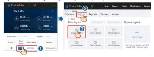
Step 2 Log in to https://intl.fusionsolar.huawei.com to access the WebUI of the FusionSolar Smart PV Management System. On the Home page, click the plant name to go to the plant page. Select Layout. Choose Generate layout, and create a physical layout as prompted. You can also manually create a physical location layout.
