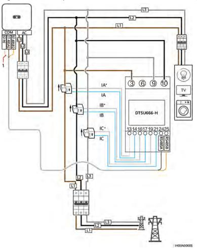
Figure 5-23 Three-phase, three-wire connection (Smart Dongle networking)
