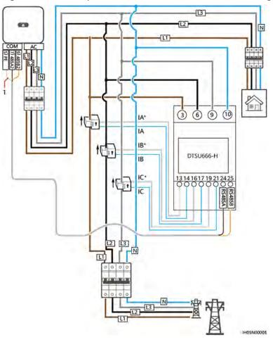
Figure 5-24 Three-phase, four-wire connection (Smart Dongle networking)
