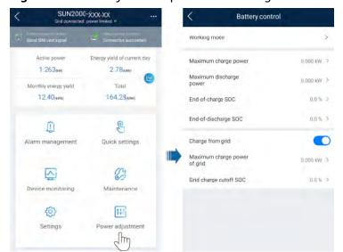
Figure 7-14 Battery control parameter setting
