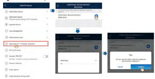
Figure 7-10 Detect optimizer disconnection
