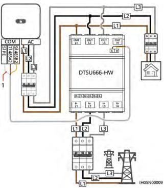
**Figure 5-25** Three-phase, three-wire direct connection (Smart Dongle networking)
