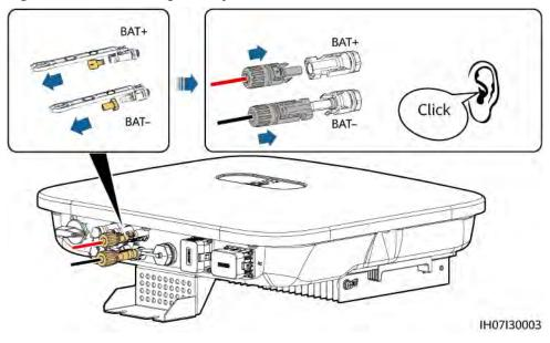
Figure 5-15 Connecting battery cables
