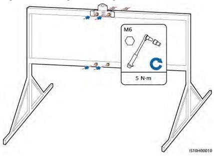
Figure 4-15 Securing the mounting bracket
