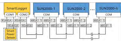
**Figure 5-20** SmartLogger networking (the dashed box indicates optional components)
