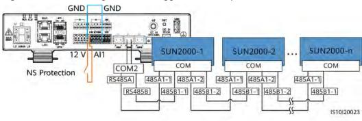
Figure 5-41 Connecting the SmartLogger to the NS protection switch
