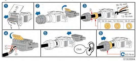
Figure 5-6 Four-core cable (L1, L2, L3, and PE)
