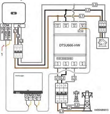
**Figure 5-27** Three-phase, three-wire direct connection (SmartLogger networking)
