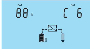
This page means SOC is 88% and battery pack units are 6.
