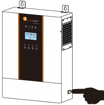
Once the unit has been properly installed and the batteries are connected well, simply press On/Off switch (located on the bottom of the case) to turn on the unit.
