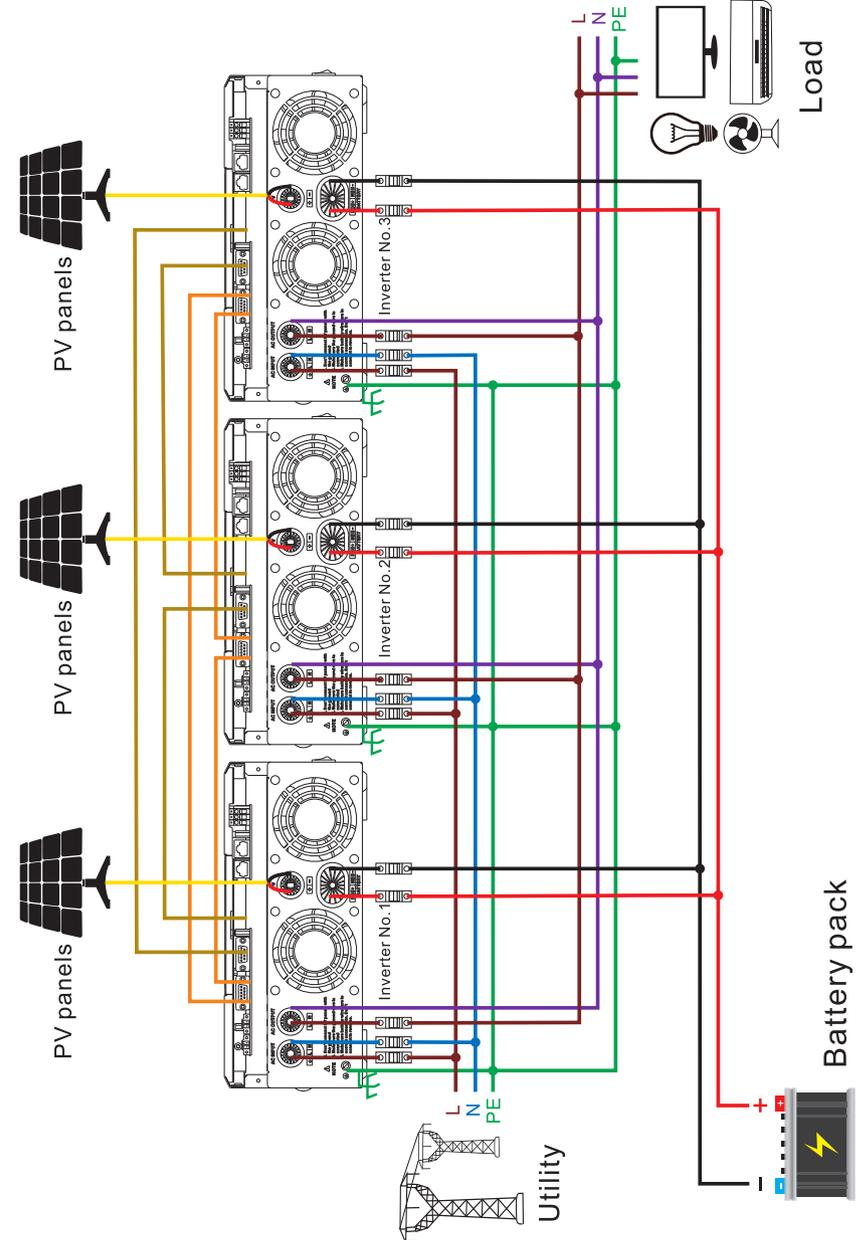
**NOTE:** Before starting up inverters, please connect all N wires of AC output together.
