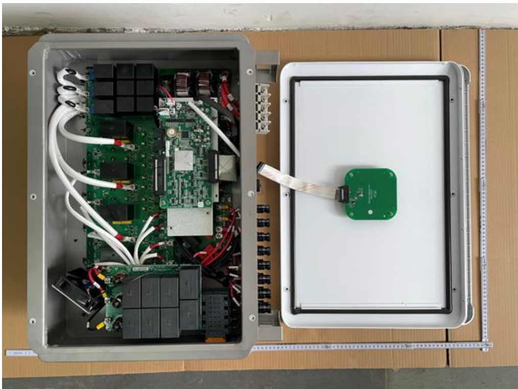
Internal view of R6-50K-T4-32, R6-40K-T4-32, R6-36K-T4-32
