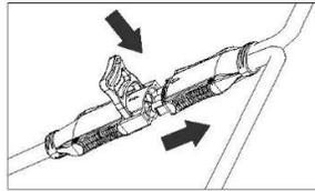
Best Practice: Use the AC Bus Cable Unlock Tool to disconnect the connectors.
