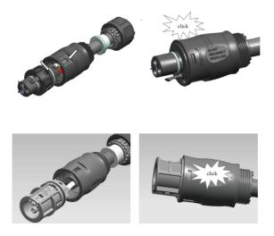
Push the sealing body and sealing craw into the housing body, and then tighten the end locker, torque  $4.0\pm0.5N$  m.
