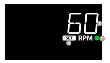
R. Speed Setting Indicator: Illuminates until stirrer reaches the Speed Setting (S).
