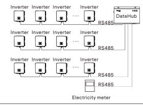
Ensure that RS485+ is connected to DataHub's RS485+ ,RS485- is connected to DataHub's RS485-, RS485 GND is connected to the GND of DataHub.
