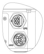
Remove the GRID connector: Press the bayonet out of the slot with a small screwdriver or the unlock tool and pull it out, or unscrew the threaded sleeve, then pull it out.
