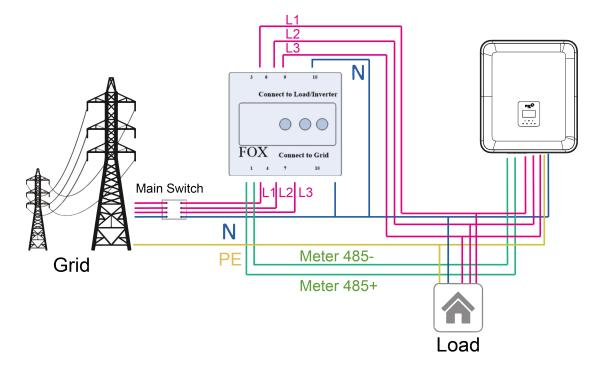
The inverter can also provide the use of two meters, using the second meter to read the power generated by another machine, where the address of the second meter is 2. When using the second meter function, you need to turn on the second meter function.
