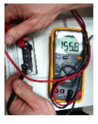
If the measured voltage deviates significantly from the nominal value, please check the electrical voltage at the individual modules, as shown in the following section.
