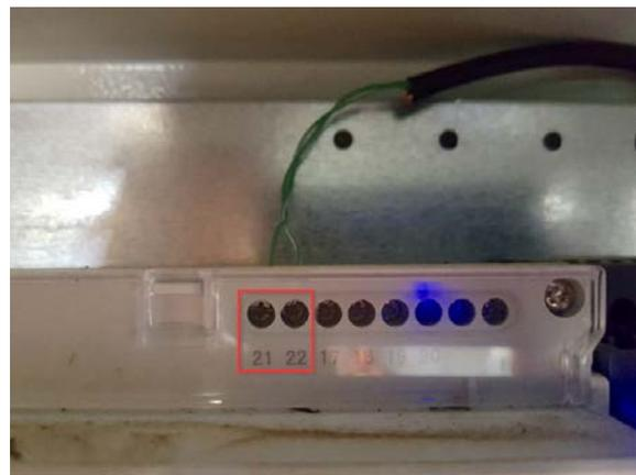
Connect to Logger1000 via the RS485 cable from the energy meter on RS485 port A2 and B2 if it has not been used.
